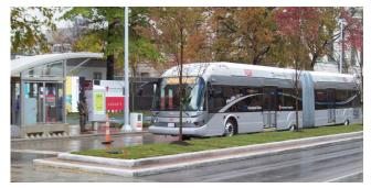
GCRTA operates a special fleet of customized New Flyer DE60LFA diesel-electric hybrid buses on the HealthLine.
