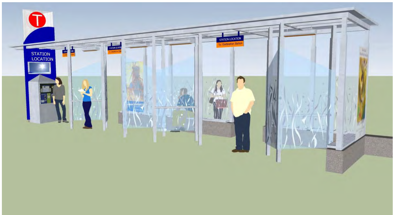
Figure 19. Large Station with Windscreen
