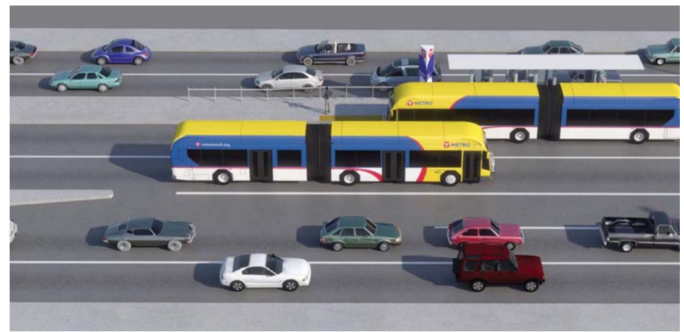
BRT in bus-only lanes
