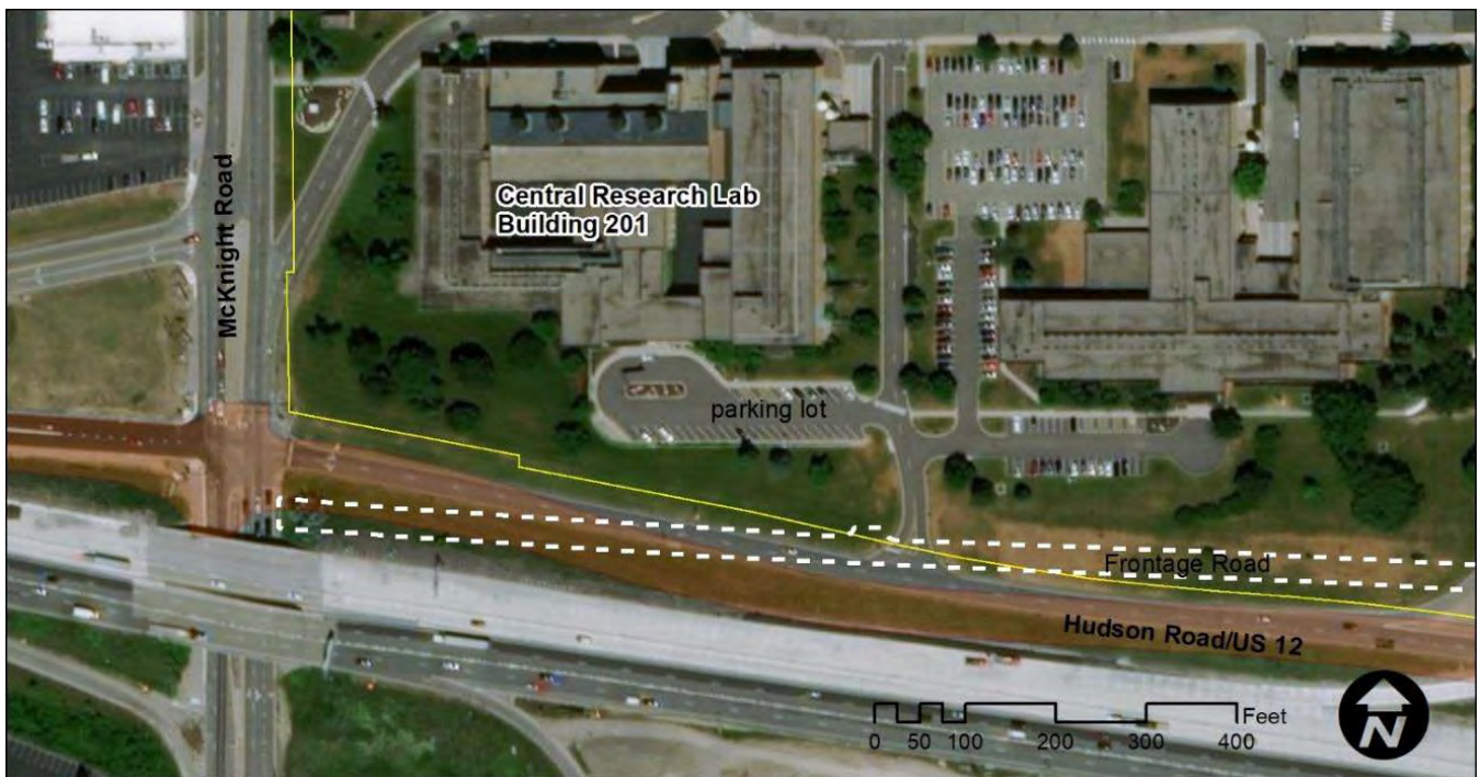
Figure 12. Intersection of McKnight Road, Hudson Road, and I-94. The orange-shaded area shows the previous alignment of Hudson Road and the white dash line shows the former frontage road, demonstrating the constant evolution of transportation corridors along the southern edge of 3M Campus Historic District.
