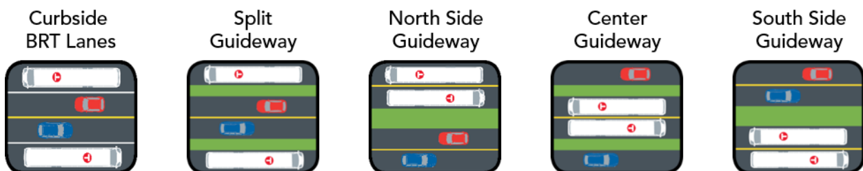
Figure 17. Guideway Configurations Considered on 4 th Street
