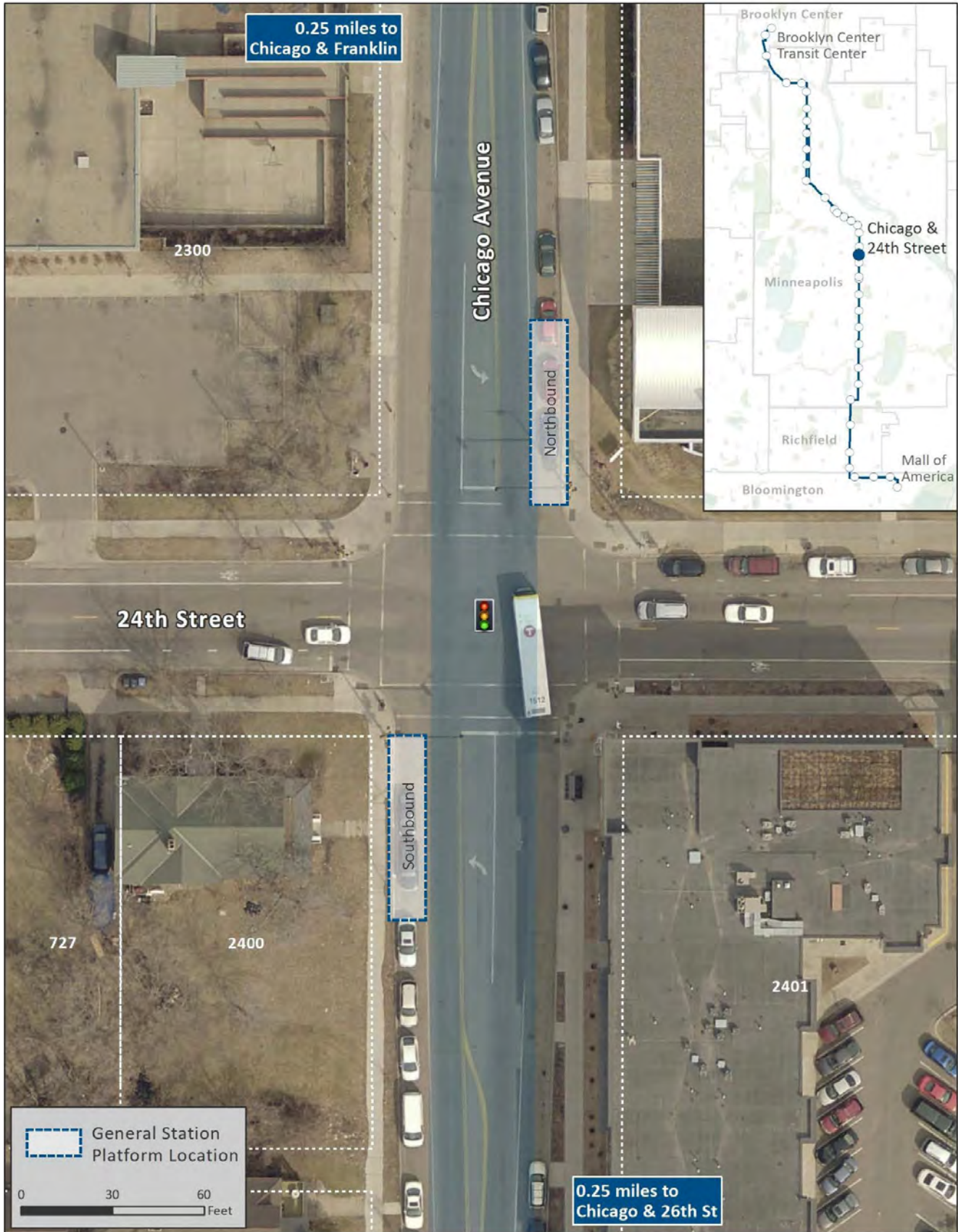
Figure 39: Recommended station location – Chicago & 24th Street
