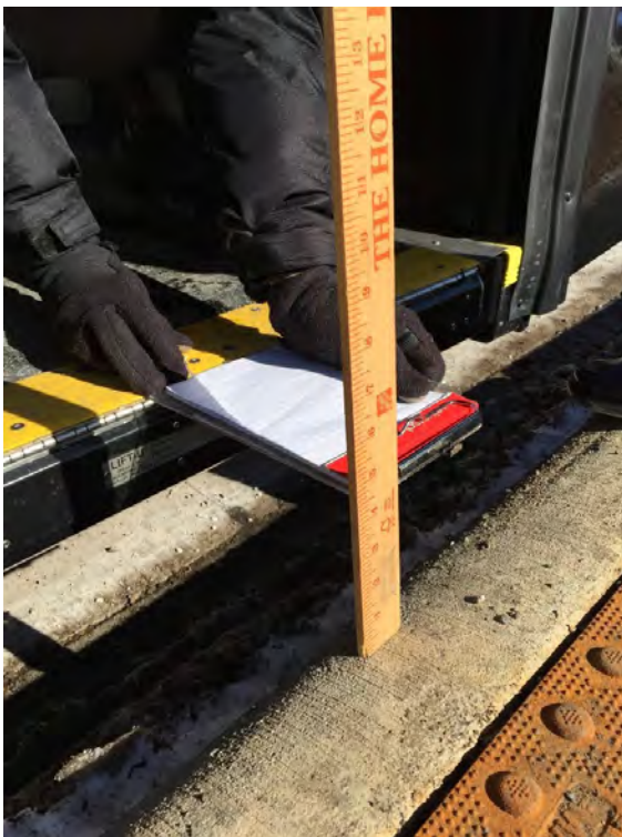
Figure 15: Near-level boarding detail
